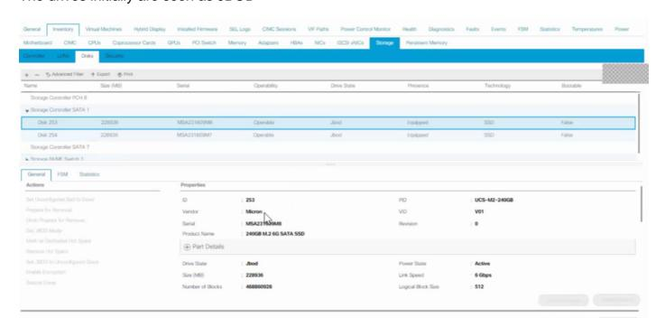
Create the storage profile for the service profile to be associated to the server, the disk group config is done manually with the disks configured in a certain RAID level, 1 being the supported one in the given construct.
