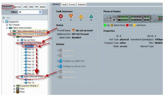
7. As shown, an Uplink Ethernet Port is successfully configured. Click **OK**.
