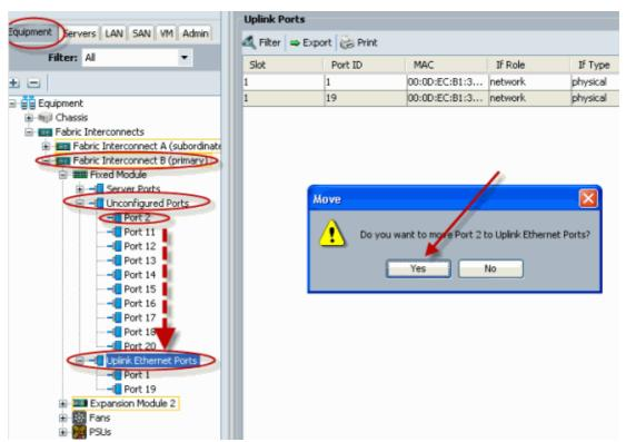
8. Make sure the new Uplink Ethernet Port is physically connected to your upstream LAN switch and the proper VLANs are configured.
