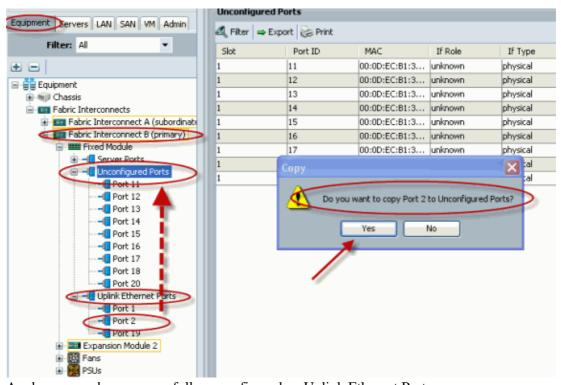
8. As shown, you have successfully unconfigured an Uplink Ethernet Port.
