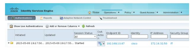
After successful authentication, the ASA-VPN creates a VPN session with the SGT tag 2 (returned in Radius Access-Accept in cisco-av-pair):
