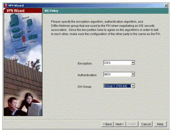
5. Provide the Encryption and Authentication parameters for the Transform Set and click Next.
