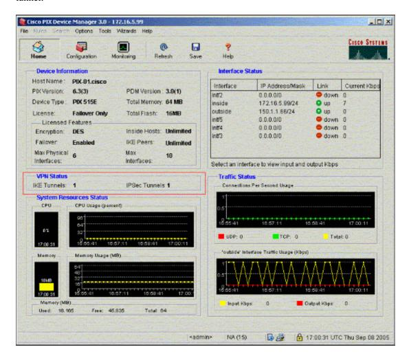
You can also verify the formation of tunnels using CLI under Tools in the PDM. Issue the **show crypto isakmp sa** command to check the formation of tunnels and issue the **show crypto ipsec sa** command to observe the number of packets encapsulated, encrypted, and so forth.
