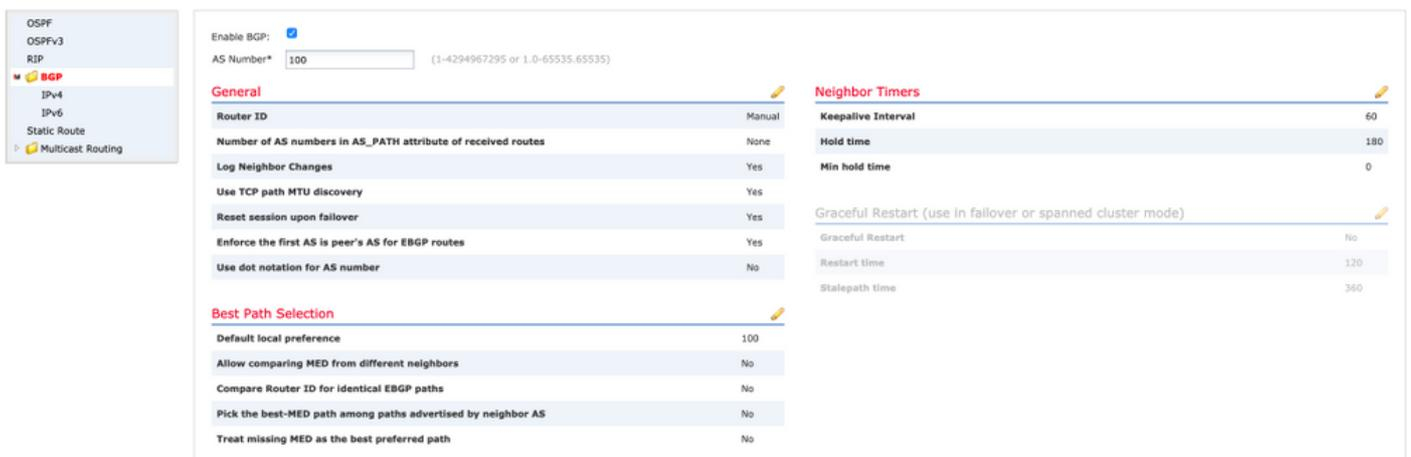
2. Navigate to **BGP > IPv4** and enable BGP IPv4 on the FTD, as shown in this image.
