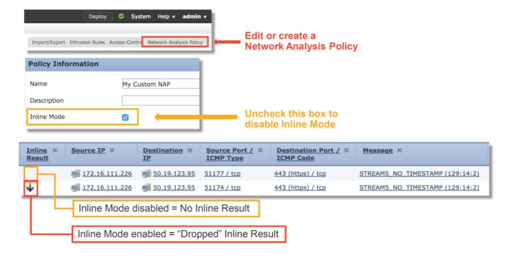
As seen in the illustration above, the NAPs contain an "Inline Mode" feature, which is the equivalent of the "Drop When Inline" option in the Intrusion Policy. A quick mitigation step for preventing the NAP from dropping traffic would be to uncheck **Inline Mode**. The Intrusion Events generated by the NAP don't display anything in the **Inline Result** tab with **Inline Mode** disabled.
