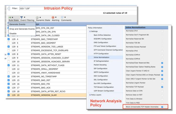
Turning on the GID 129 rules causes Intrusion Events to be sent to the FMC when they take action on the traffic. However, as long as the **Block Unresolvable TCP Header Anomalies** is enabled, it can still drop traffic even if the **Rule State** in the Intrusion Policy is set to only **Generate Events**. This behavior is explained in the FMC Configuration Guides.
