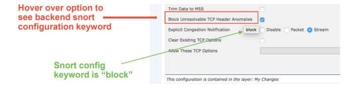
The **Block Unresolvable TCP Header Anomalies** option in the NAP tab translates to the **block** keyword on the backend. With that information in mind, the backend configuration can be checked
