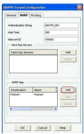
2. Depending on the network setup, NHRP mapping parameters can be configured as shown here:
