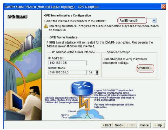
6. Verify the tunnel parameters and NHRP parameters, and make sure they match perfectly to the Hub parameters.
