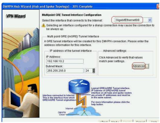
6. Specify the Tunnel parameters and NHRP parameters. Then, click OK.
