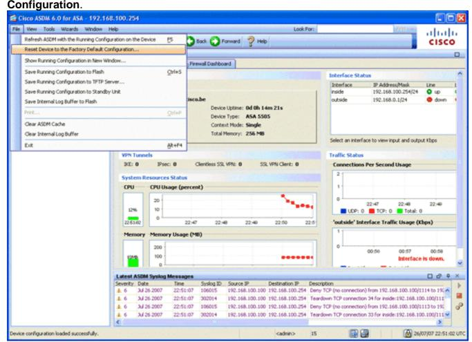
Leave the default values in the template. Connect your PC on the Ethernet 0/1 inside interface, and renew your IP address that will be provisioned by the DHCP server of the ASA. **Note:** In order to reset the ASA to the factory defaults from the command line, use these commands
