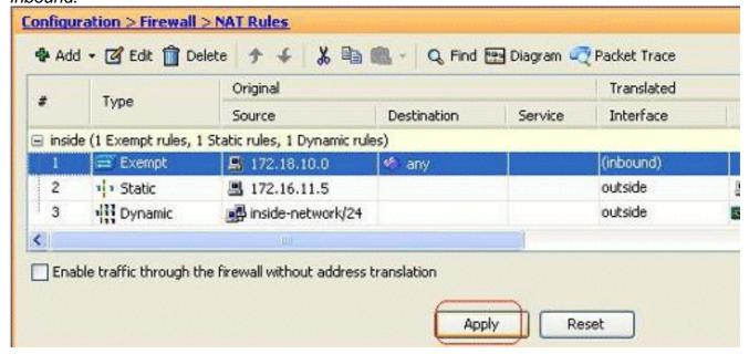
Click Apply in order to send this CLI output to the ASA:  $access-list inside_nat0_outbound extended permit ip host 172.18.10.0 any$
