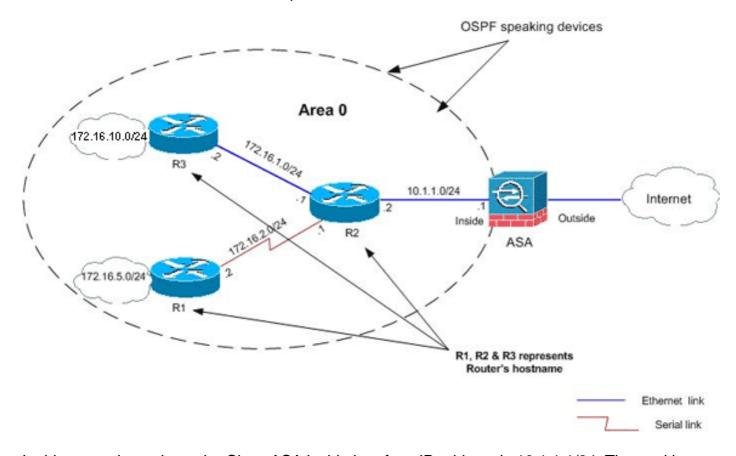
In this network topology, the Cisco ASA inside interface IP address is 10.1.1.1/24. The goal is to configure OSPF on the Cisco ASA in order to learn routes to the internal networks (172.16.1.0/24, 172.16.2.0/24, 172.16.5.0/24 and 172.16.10.0/24) dynamically through the adjacent router (R2).
