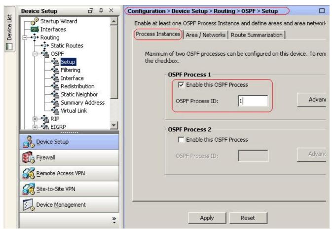
4. You can click **Advanced** on the **Setup > Process Instances** tab in order to configure optional advanced OSPF routing process parameters. You can edit process-specific settings, such as the Router ID, Adjacency Changes, Administrative Route Distances, Timers, and Default Information Originate settings.
