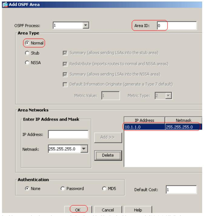
In this example, the only network that is added is the inside network (10.1.1.0/24) since OSPF is enabled only on the inside interface. **Note:** Only interfaces with an IP address that fall within the defined networks participate in the OSPF routing process.
