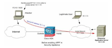
Unicast RPF can prevent attacks based on source address spoofing. You need to configure the uRPF in the outside interface of the ASA as shown here:
