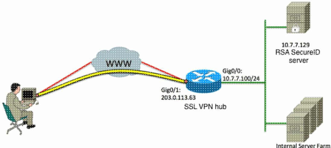
One of the differences between the Adaptive Security Appliance (ASA) and Cisco IOS headends is that Cisco IOS Router/switches/Access Points (APs) only support RADIUS and TACACS. They do not support the RSA-proprietary protocol SDI. The RSA server however supports both SDI and RADIUS. Therefore, in order to use OTP authentication on a Cisco IOS headend, the Cisco IOS device must be configured for RADIUS protocol and the RSA server as a RADIUS token server.
