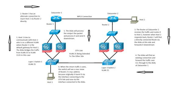
For an Inter Domain Controller (DC) communication in transparent mode, this specific traffic flow is not covered or documented but this specific traffic flow does work from an ASA flow processing standpoint. However, it can result in MAC move notifications on the switch.
