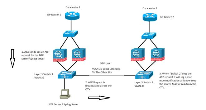
This specific case will be observed for any traffic which gets generated by the ASA itself. Here two possible situations are considered, wherein the ASA either tries to reach an Network Time Protocol (NTP) or a Syslog server, which are on the same subnet as that of its BVI interface. However it is not only limited to these two conditions, this situation can happen whenever traffic is generated by the ASA for any IP address which is directly connected to the BVI IP addresses.
