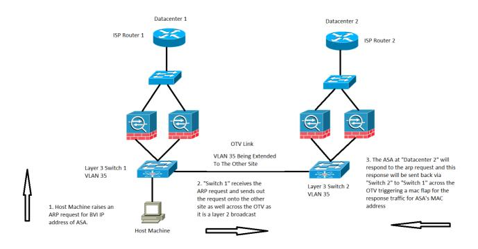
A MAC MOVE can also be observed at times when traffic is destined to the ASA's BVI IP address.
