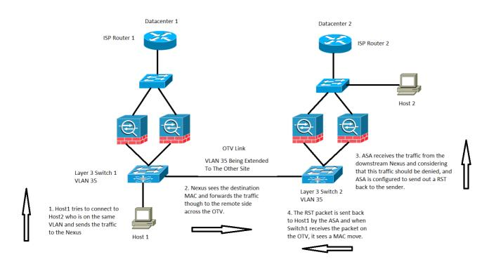
In this case, we have a host Host 1 on VLAN 35, it tries to communicate with Host 2 in the same Layer 3 VLAN, however, Host 2 is actually on Datacenter 2 VLAN 1535.
