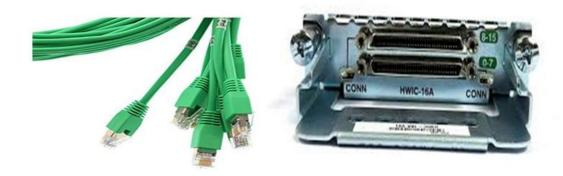
A close look at the cables indicates a number in a pattern of P0, P2,....P7 and on the card for the top port the number is from 8 - 15 and the bottom one is from 0 - 7. Based on the diagram mentioned, you can say that, for R1 you use line 0/0/0, for R2 line 0/0/1, for R3 line 0/0/8 and for R4 0/0/9.
