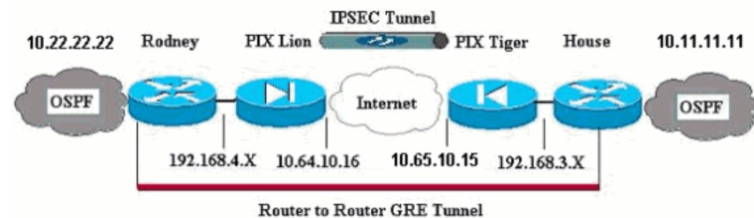
**Note:** The IP addressing schemes used in this configuration are not legally routable on the Internet. These are RFC 1918 [addresses](#) which have been used in a lab environment.
