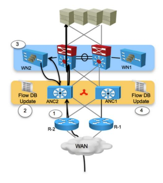
Step 1. ANC2 receives a TCP SYN packet from one of the branches that contain a WAAS device.
