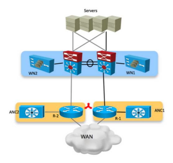
In an Active/Active WAN router (Core Switch) environment, traffic is forwarded by different devices based on their routing configuration. For some connections packets that reach the server (incoming flow) and packets that leave from the server (outgoing flow) hit the same router. There can be some connections, where different routers handle the packets that come toward the server and packets that leave from the server.
