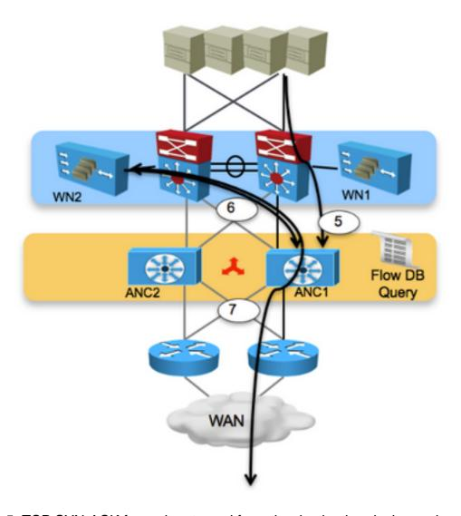
Step 5. TCP SYN-ACK frame is returned from the destination device and goes to ANC1.
