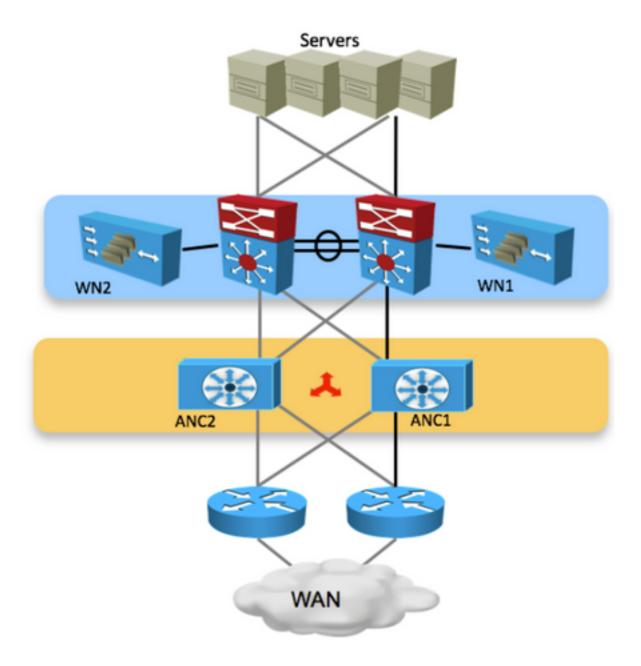
This image shows APPNAV-XE component where ANC is inside the router. Each ANC and WN in the cluster have IP connectivity and reachability between them.
