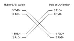
The table below lists the pinouts for the Ethernet RJ-45 crossover cable.
