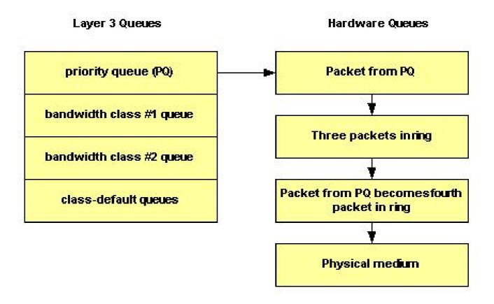
Use the tx-ring-limit command to tune the size of the transmit ring to a non-default value. Cisco recommends that you tune the transmit ring when you transmit voice traffic.
