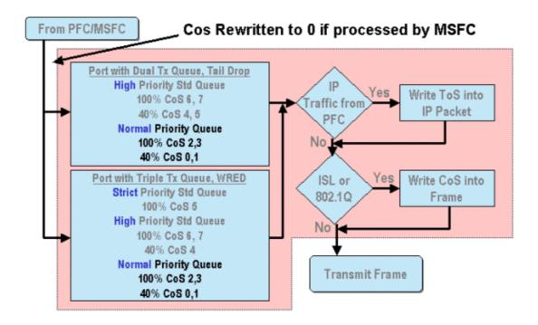
When a frame is processed by either the MSFC or the PFC, it is passed to the outbound port ASIC for further processing. Any frames processed by the MSFC will have their CoS values reset to zero. This needs to be taken into consideration for QoS processing on outbound ports.
