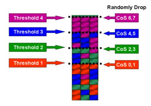
The above figure shows an input queue with four thresholds, and how COs values have been assigned to each threshold.
