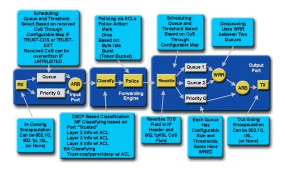
A frame enters the switch and is initially processed by the port ASIC that received the frame. It will place the frame into a Rx queue. Depending on the Catalyst 6000 family line card, there will be one or two Rx queues.
