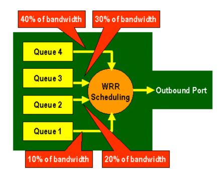
On the WS-X6248 and WS-X6348 line cards (with 2q2t queue structures), two TX queues are used by the WRR mechanism for scheduling. On the WS-X6548 line cards (with a 1p3q1t queue structure) there are four TX queues. Of these four TX queues, three TX queues are serviced by the WRR algorithm (the last TX queue is a SP queue). On GE line cards, there are three TX queues (using a 1p2q2t queue structure); one of these queues is a SP queue so the WRR algorithm only services two TX queues.
