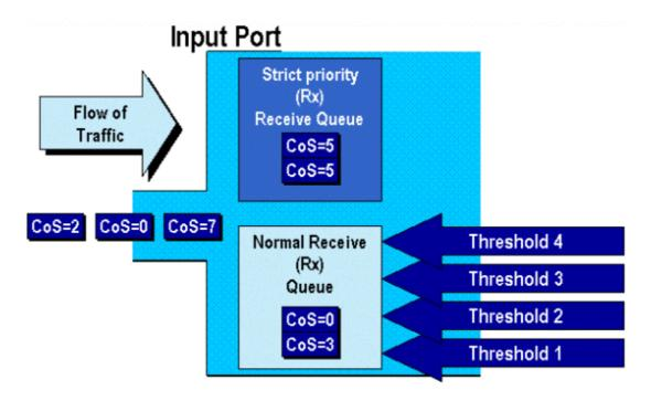
As shown in the above diagram, frames arrive and are placed in the queue. As the queue starts to fill, the thresholds are monitored by the port ASIC. When a threshold is breached, frames with COs values identified by the administrator are dropped randomly from the queue. The default threshold mappings for a 1q4t queue (found on WS-X6248-RJ45 and WS-X6348-RJ45 line cards) are as follows:
