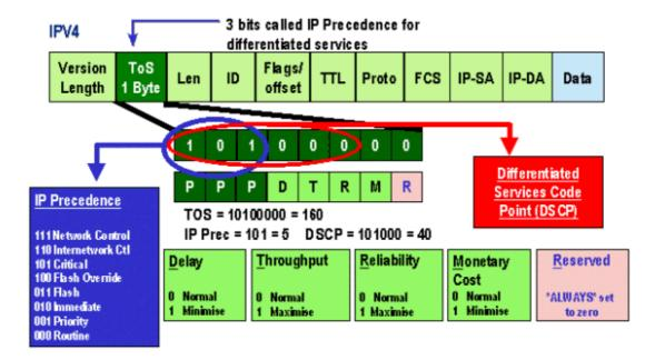
More recently, the use of the ToS field has been expanded to encompass the six MSBs, referred to as DSCP. DSCP results in 64 priority values (two to the power of six) that can be assigned to the IP packet.
