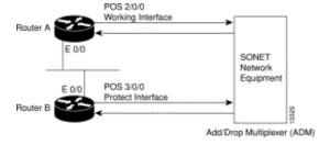
Use this configuration on router A, which contains the working interface:
