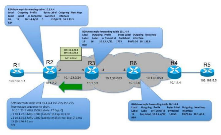
R3 will reply back to R2 with MPLS Echo Reply with DSMAP TLV carrying outgoing label 16 and additional information like downstream neighbor details. Unlike ICMP messages, MPLS Echo Reply will be directly forwarded from responder R3 to Initiator R2.
