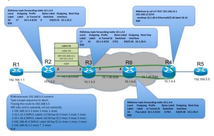
R3 will buffer the label stack and generate ICMP error message and include the incoming label stack from the buffer in ICMP payload. It further populate the IP header with source address from incoming interface of the labeled packet, destination address as the source of the labeled packet. The TTL is set to 255. It now pushes the label stack from the buffer and consults the LFIB table for
