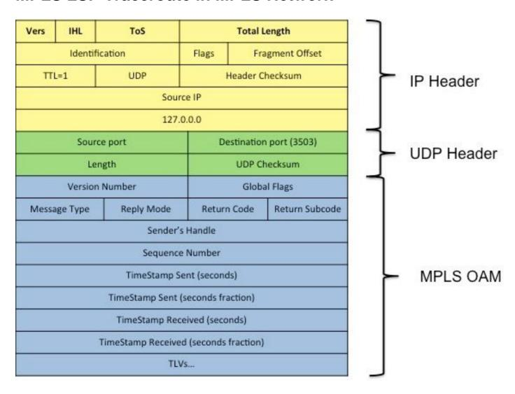
Unlike ICMP based traceroute, LSP traceroute uses the machinery defined in RFC4379. It uses IP/UDP encapsulation with destination address of request set to loopback address (127.0.0.0/8 range). It is expected that LSP Ping is to be triggered within the same MPLS domain and so reply will be directly sent to the Initiator.
