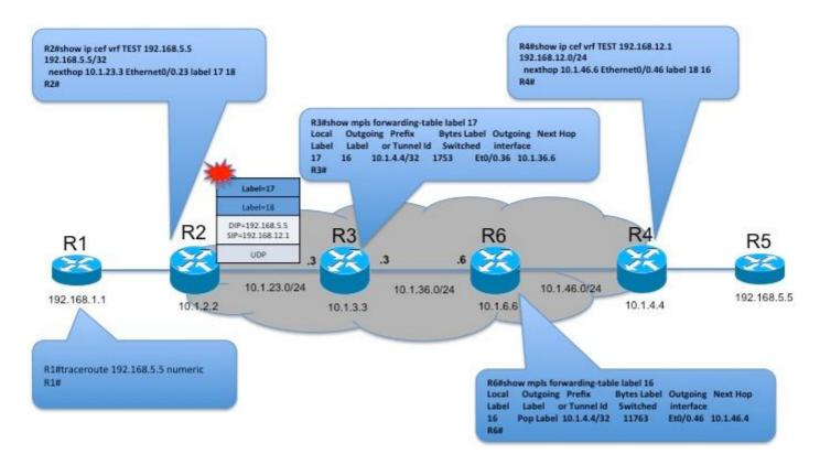
In this topology, when ICMP traceroute is triggered from R1 (CE) to 192.168.5.5 (remote CE), the first packet is sent with TTL of 1. This is normal IP packet and so R2 follows the traditional behavior of generating ICMP and sending directly to R1. The second packet sent with TTL=2 will expire at R3.
