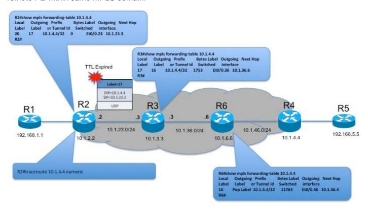
In this topology, when ICMP traceroute is triggered from R2 to 10.1.4.4, the first packet is sent with TTL of 1. R3 on receiving the packet will decrement the TTL to 0 and trigger ICMP generation mechanism.
