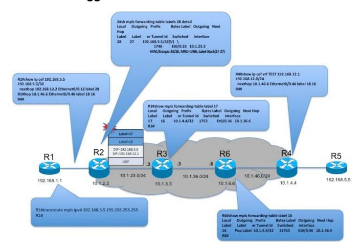
This is applicable in CSC like scenarios where MPLS is enabled between PE-CE. There are 2 challenges in executing LSP trace from CE to remote CE over Carrier MPLS domain as below:
