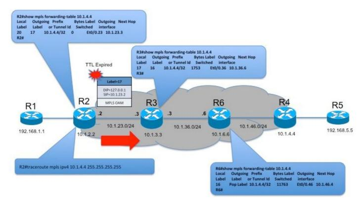
In this topology, LSP trace is triggered from R2 to validate the LSP to prefix 10.1.4.4/32. The TTL on the label will be set from 1. R3 on receiving it will punt to CPU for OAM processing.
