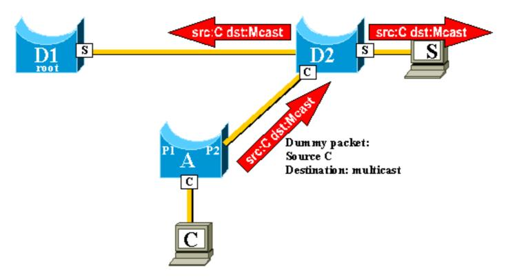
The rate at which the dummy multicasts are sent can be configured.
