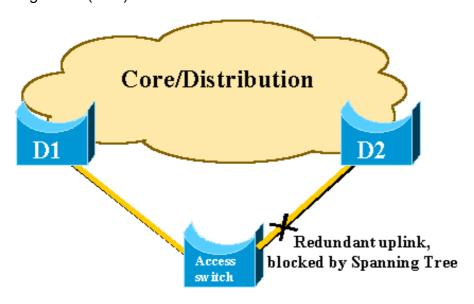
In the event of failure of the primary uplink to core switch D1, the STP recalculates and eventually unblocks the second uplink to switch D2, therefore it restores connectivity. With the default STP parameters, the recovery takes up to 30 seconds, and with aggressive timer tuning, this lapse of time can be reduced to 14 seconds. The UplinkFast feature is a Cisco proprietary technique that reduces the recovery time further down to the order of one second.
