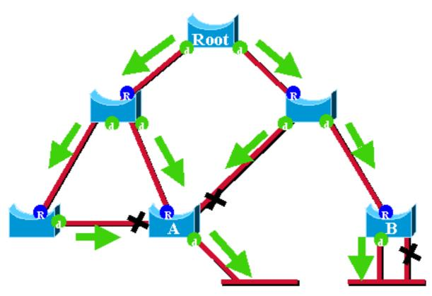
In this diagram, root ports are represented with a blue R and designated ports are represented with a green d. The green arrows represent the BPDUs generated by the root bridge and retransmitted by the bridges on their designated ports. Without the entrance a formal demonstration, you can determine these about BPDUs and ports in a stable network:
