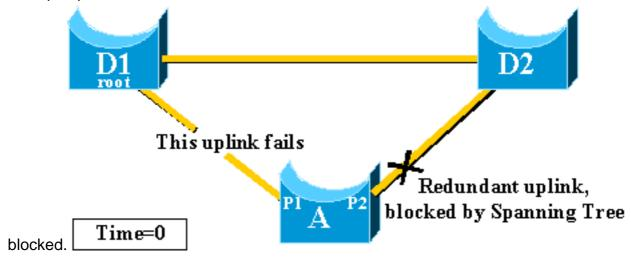
3. A places port P2 in forwarding mode immediately, thus it violates the standard STP procedures. There is no loop in the network, as the only path to the root bridge is currently down. Therefore, recovery is almost immediate.
