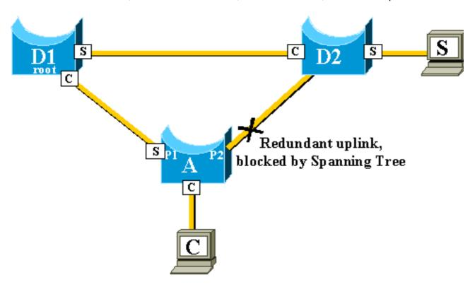
The CAM tables of the different switches are represented in the diagram. You can see that, in order to reach C, packets originated from S have to go through D2, D1, and then A.
