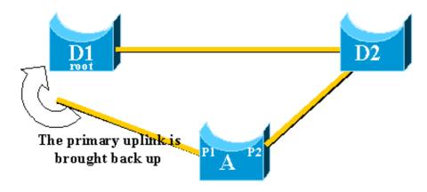
No. An immediate switchover to port P1, which immediately blocks port P2 and put port P1 in forwarding mode, is not wanted, for these reasons:
