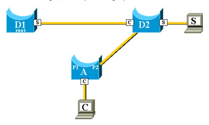
The backup link is brought up so quickly, however, that the CAM tables are no longer accurate. If S sends a packet to C, it is forwarded to D1, where it is dropped. Communication between S and C is interrupted as long as the CAM table is incorrect. Even with the <u>topology change mechanism</u>, it can take up to 15 seconds before the problem is solved.
