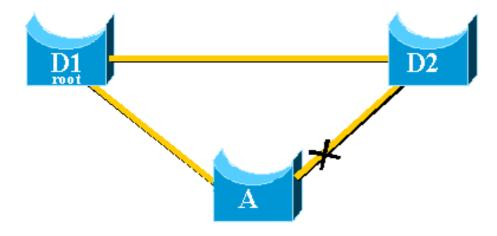
Switches A, D1, and D2 are all Catalyst switches that support the UplinkFast feature. Focus on switch A, while you perform these steps:
