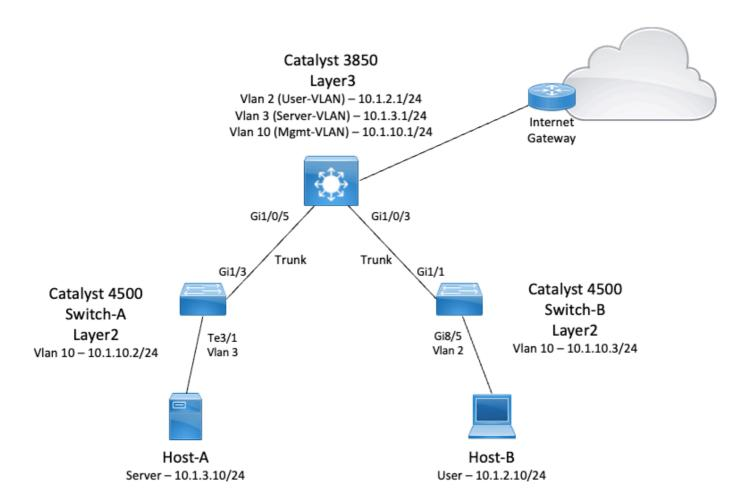
In this diagram, a small sample network with the Catalyst 3850 provides Inter VLAN routing between the various segments. The Catalyst 3850 switch can act as an L2 device with the disablement of IP routing. In order to make the switch function as an L3 device and provide Inter VLAN routing, make sure that ip routing is enabled globally.
