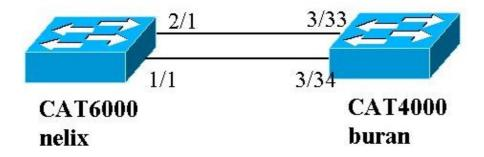
In this example, we configure an LACP aggregate link between a Catalyst 4000 and Catalyst 6000 series switch using two Gigabit Ethernet ports as shown in the diagram above.
