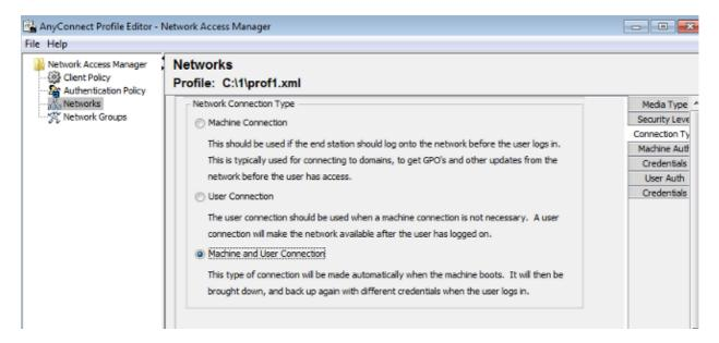
Then, it is possible to configure separate authentications from the Machine Authentication and User Authentication tabs.
