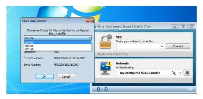
When the test2 certificate is used, the switch receives a success response along with the RADIUS attributes.
