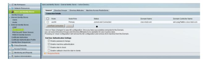
ACS matches AD usernames with the use of the CN field from the certificate received from the supplicant (in this case it is test1, test2, or test3). Binary comparison is also enabled. This forces ACS to obtain the user certificate from AD and compare it with the same certificate received by the supplicant. If it does not match, authentication fails.
