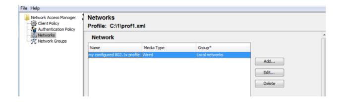
At this stage it is very important is to give the user the choice to use the certificate at each authentication. Do not cache that choice. Also, use the 'username' as the unprotected id. It is important to remember that it is not the same id which is used by ACS to query AD for the certificate. That id will be configured in ACS.
