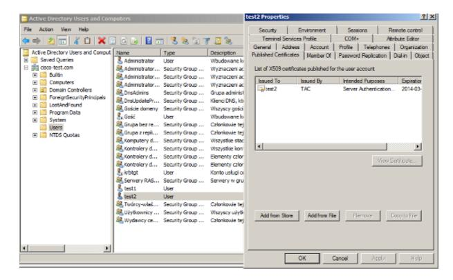
At this stage, the certificate is binded to a specific user in AD. This can be verified with the use of ldapsearch:
