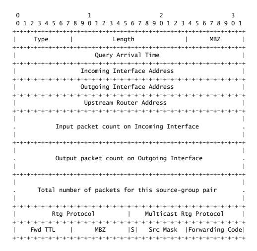
It is this response block information that is used to display the traceroute output. Each response block is one line in the mtrace output.
