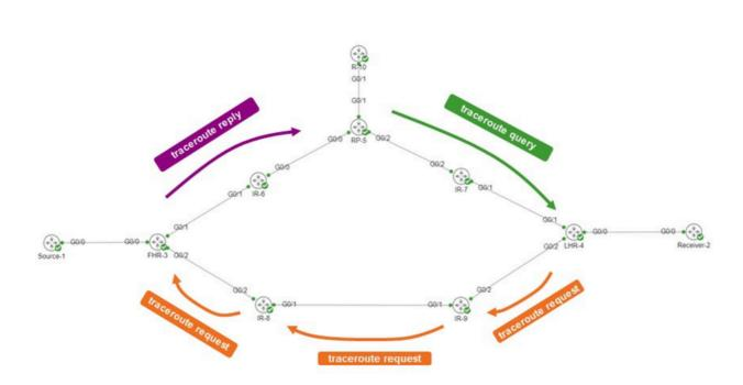
The originator is R-10. The LHR is LHR-4. The FHR is FHR-3. The RP is RP-5. The network is running PIM Sparse mode or Any Source Multicast (ASM).
