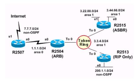
The R2513 router, which only runs RIP (and may be connected to a RIP—only network), is added to the Token Ring network in the figure. When the routes learned from R2513 are redistributed into OSPF by the ASBR (R2515), some of the routes are not installed into the routing table of some of the routers. The relevant configuration information of each of the routers is given in these tables.
