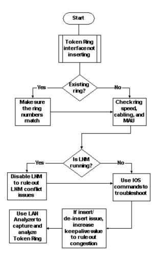
One of the first things that must be checked, when a Token Ring interface has problems with insertion into the ring, is whether or not you are inserting into a ring that already exists. If yes, you need to match the ring number configured on the Token Ring interface with the existing ring number governed by other Source–Route Bridges (SRBs).
