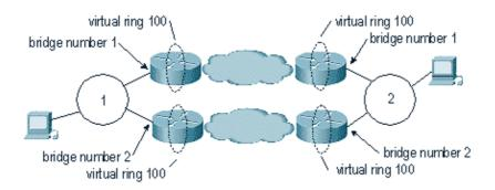
When there are multiple paths to the same ring coming from another ring, each bridge must have a different bridge number. The scenario shown in the diagram above is most common in environments with DLSw+ and
