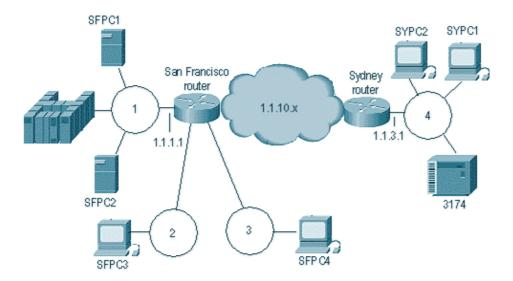
In the diagram above, station SFPC4 sends an explorer to reach SFPC1. The router will fast—switch the explorer to rings 1 and 2. But the router will also send the explorer to the explorer queue for RSRB processing to send the frame to the remote site (this is assuming that **netbios enable name cache** and **proxy explorer** commands are turned off).
