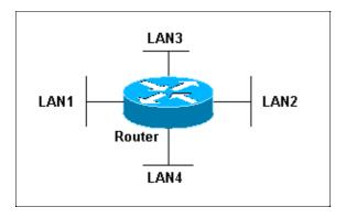
In this example, the router acts as two different bridges, one between LAN1 and LAN2, and one between LAN3 and LAN4. Frames from LAN1 are bridged to LAN2, however, not to LAN3 or LAN4, and vice versa. In other words, frames are bridged only among interfaces in the same group. This grouping feature is commonly used to separate networks or users.
