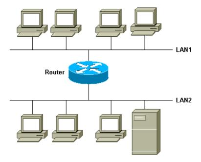
In this example, there are several PCs on LAN1, which is located on one floor. LAN2 also has many PCs and some servers, but it is on a different floor. The systems on each LAN use either IP, IPX, or DECNET. Most of the traffic can be routed, but there are some application systems that were developed with proprietary protocols and can't be routed. This traffic (such as NetBIOS and LAT) must be bridged.
