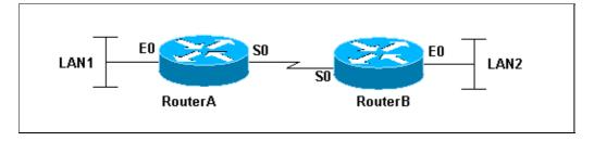
In this example, the two LANs are connected by a T1 link.
