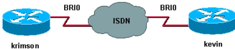
In this example, we are using two Cisco 2500 routers with BRI lines.
