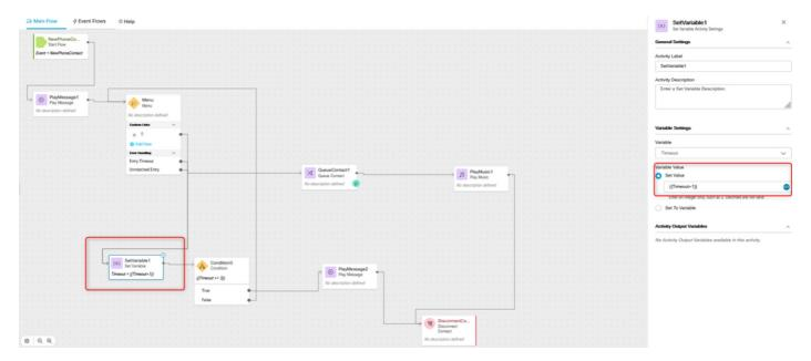
3. Configure Condition block with expression  $\{\{\text{Timeout} >= n\}\}$ , where n is the number of times you would like to return the call back to menu before the call disconnects. For example,  $\{\{\text{Timeout} >= 3\}\}$  configuration returns the call back to menu 3 times before the call disconnects as per the flow logic.
