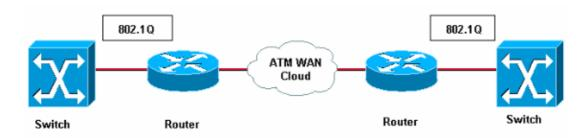
However, there is an alternate way to build end-to-end VLANs. Configure both routers with the same set of bridge groups and 802.1Q subinterfaces. In other words, the two router ends have a one-to-one mapping between a bridge-group and an 802.1Q subinterface. This is not applicable to the Cisco 7600.
