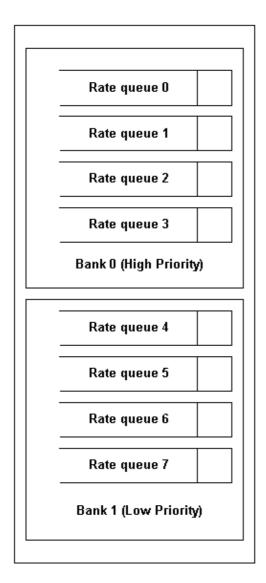
Packets linked to rate queues in the low-priority bank (bank one) cannot transmit while the rate queues in the high-priority bank (bank zero) are not empty.
