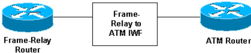
Section 5 of the FRF.8 agreement discusses two modes of upper-layer protocol encapsulation. This encapsulation refers to the header that identifies the protocol carried within the protocol data unit (PDU), allowing the receiver to properly process the incoming packet. FRF.8 defines two modes – translation and transparent. Selecting one of these modes at the interworking function determines the encapsulation we need to configure on our ATM endpoint.
