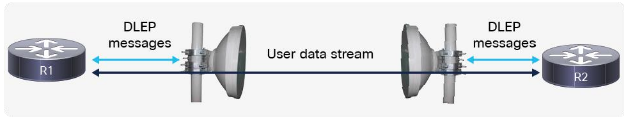
Figure 3. A radio link that implements DLEP between the router and its radio modem
