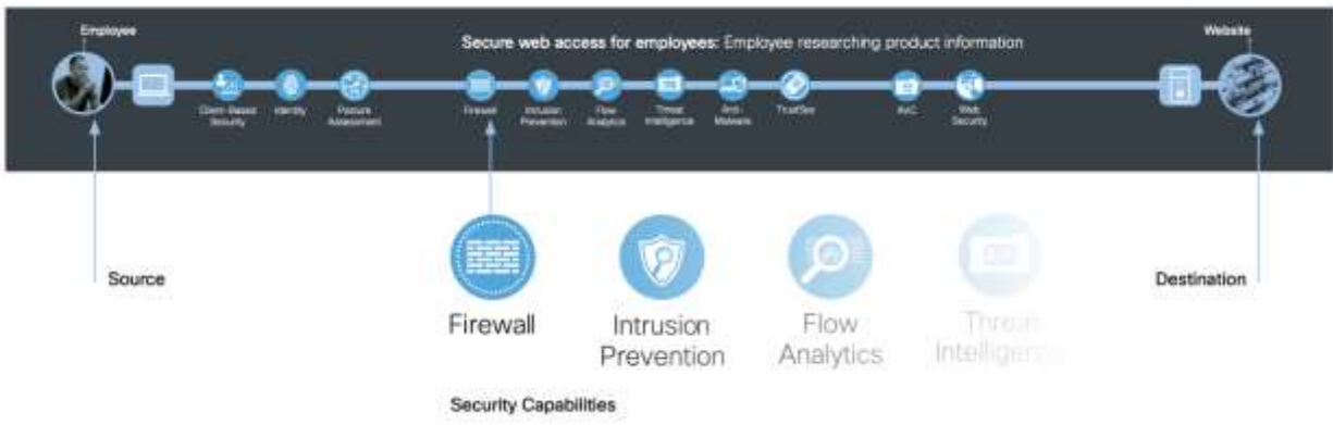
Figure 10. Business Flow with Required Security Capabilities
