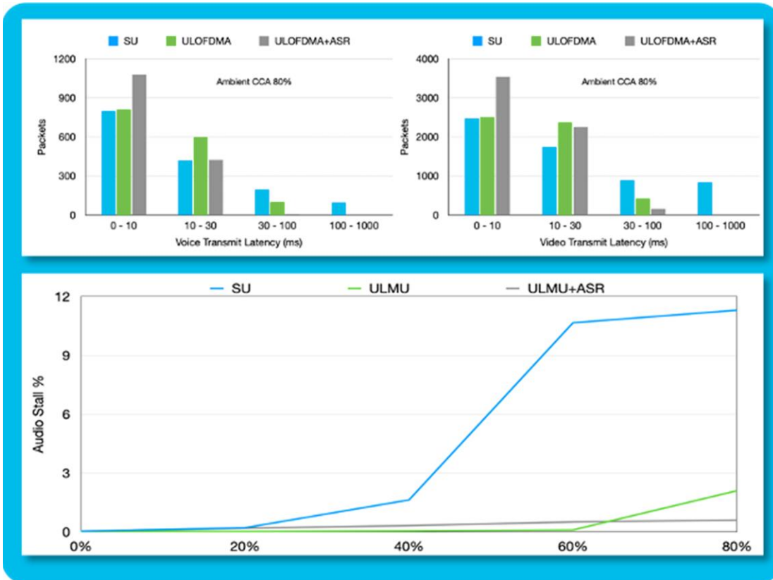
Figure 4. Fastlane+ enabled vs. disabled comparing latency (Fastlane+ is referred to as ASR)
