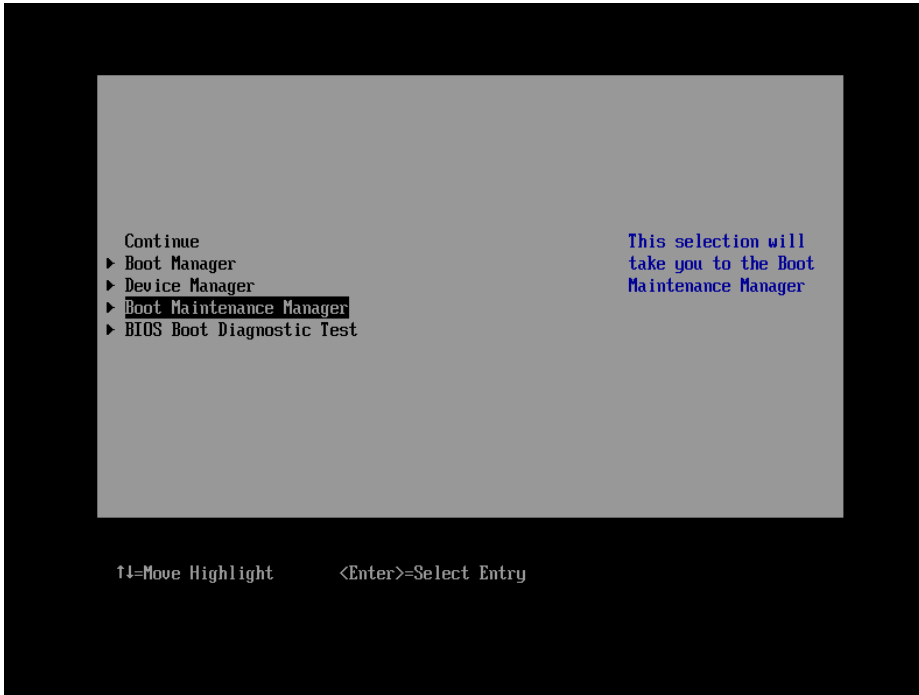
Figure 55. Selecting Boot Maintenance Manager
