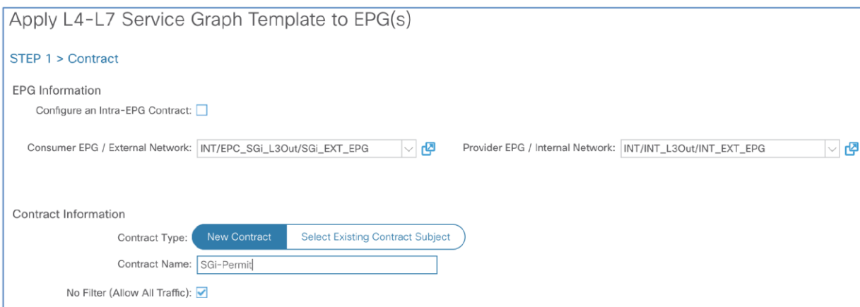
Figure 80. Screenshot from APIC to apply contract between EPGs to perform service chaining
