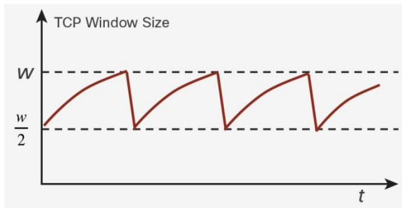
Figure 9. TCP Window-Size Dynamics for Congestion Avoidance
