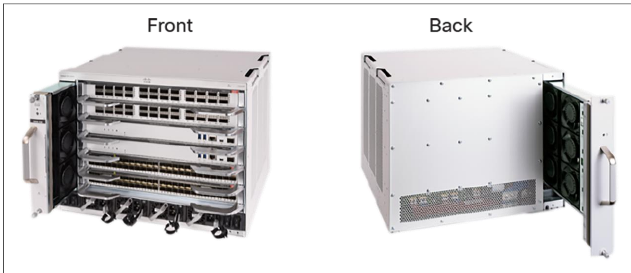
Figure 5. Flexible fan-tray servicing
