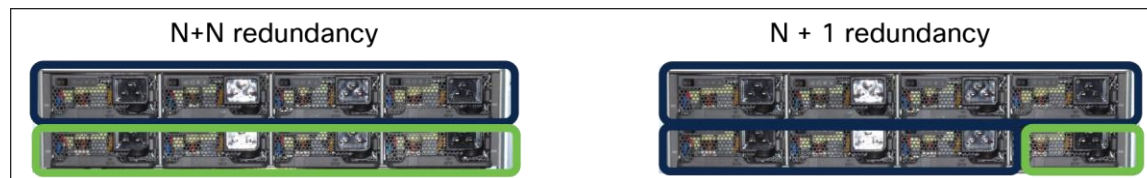
Figure 10. Power redundancy modes
