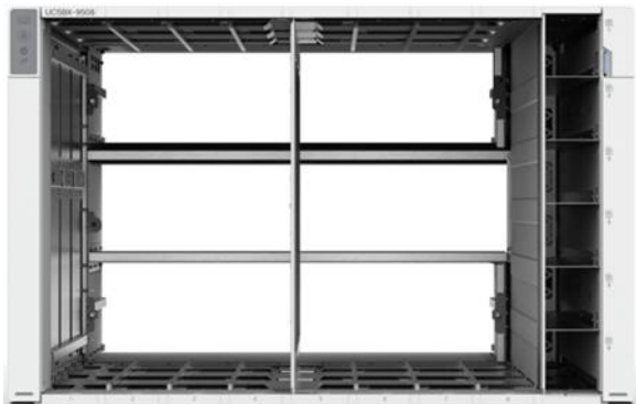
Figure 3. Cisco UCS X9508 Server Chassis: Midplane-free design
