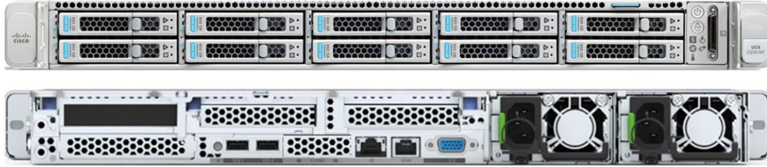
Figure 1. Front and rear view of Cisco UCS C220 M7 Rack Server
