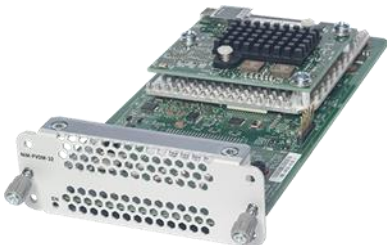
Figure 3. PVDM Network Interface Module (NIM-PVDM-X)
