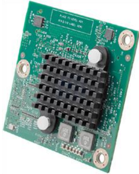
Figure 1. On-Board Motherboard PVDM (PVDM4-X)
