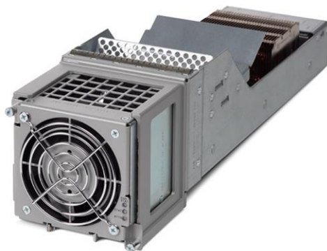
Figure 9. NCS 4009 400G Single-Chassis Fabric Line Card (NCS 4009 Fabric V2) with fan kit
