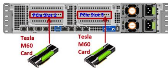
Figure 13. Two-GPU Scenario with Cisco UCS C240 M4
