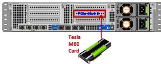
Figure 13. Two-GPU Scenario with Cisco UCS C240 M4
