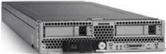
Figure 7. Cisco UCS B200 M4 Blade Server Front View
