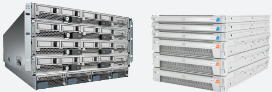
Figure 1. Cisco HyperFlex systems with both compute and storage and compute-only nodes
