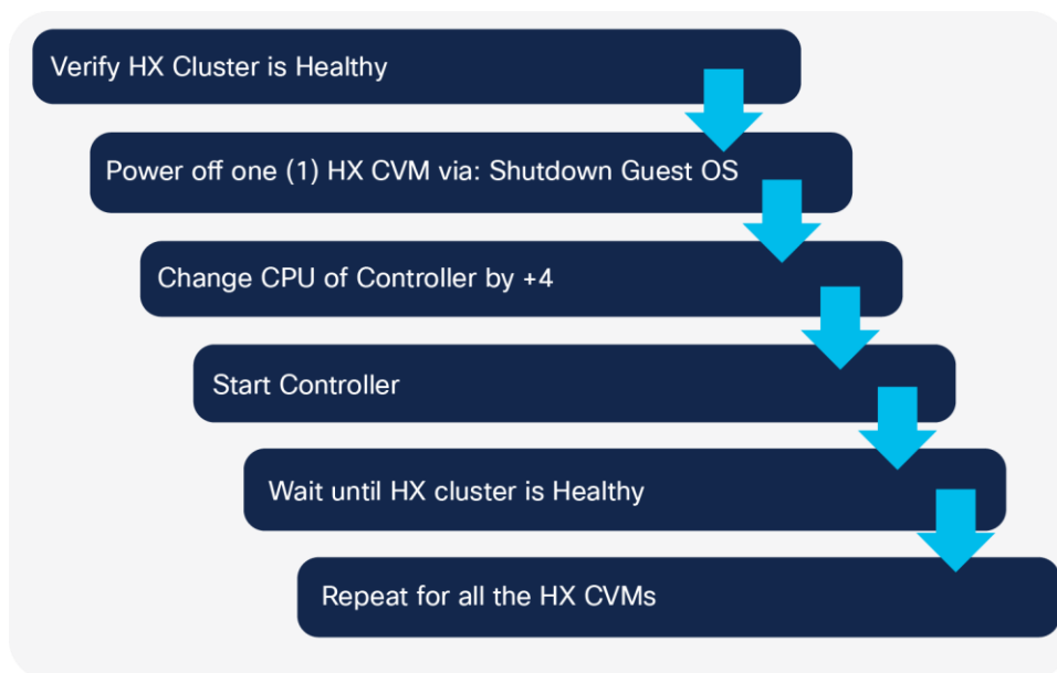
Figure 2. Workflow to enable HyperFlex Boost mode
